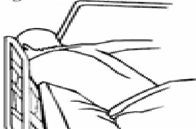
Zone 6 - Entrapment between rail end and edge of head/foot board
