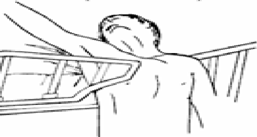
Zone 5 - Entrapment between split rails
